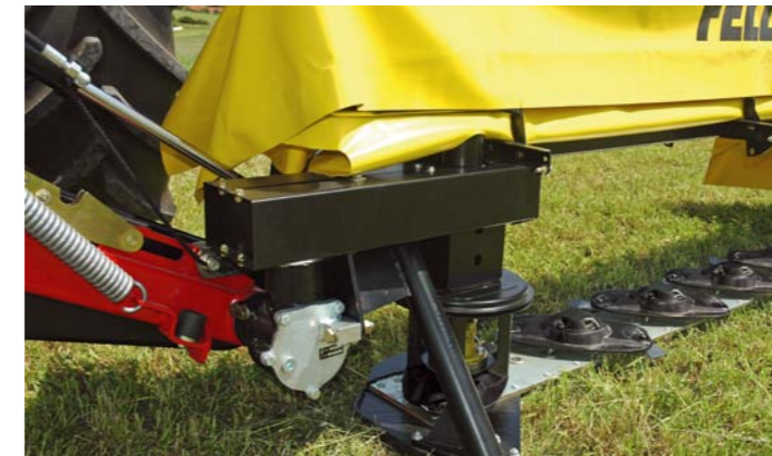
Mower without inner skid: Drive in the first mower disc
